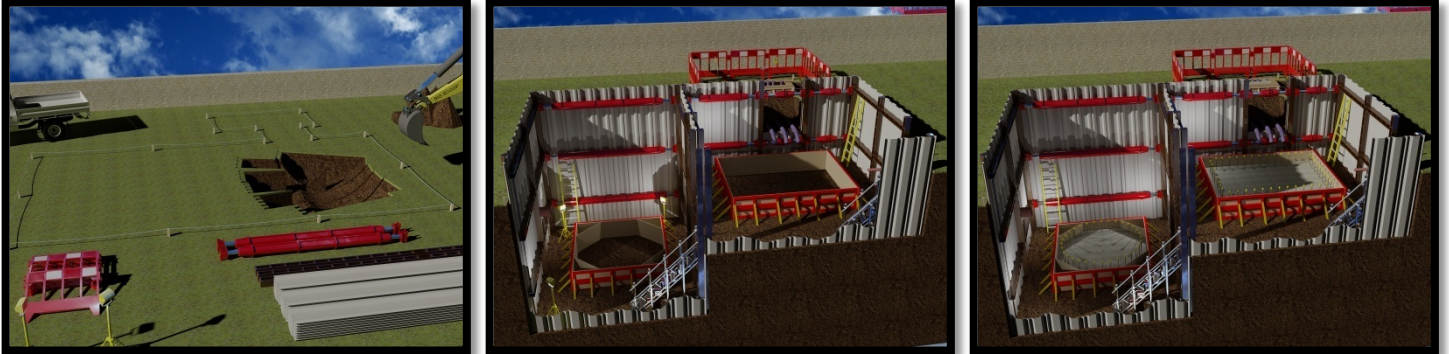
Initial site preparation, excavation and pouring of base slabs.
