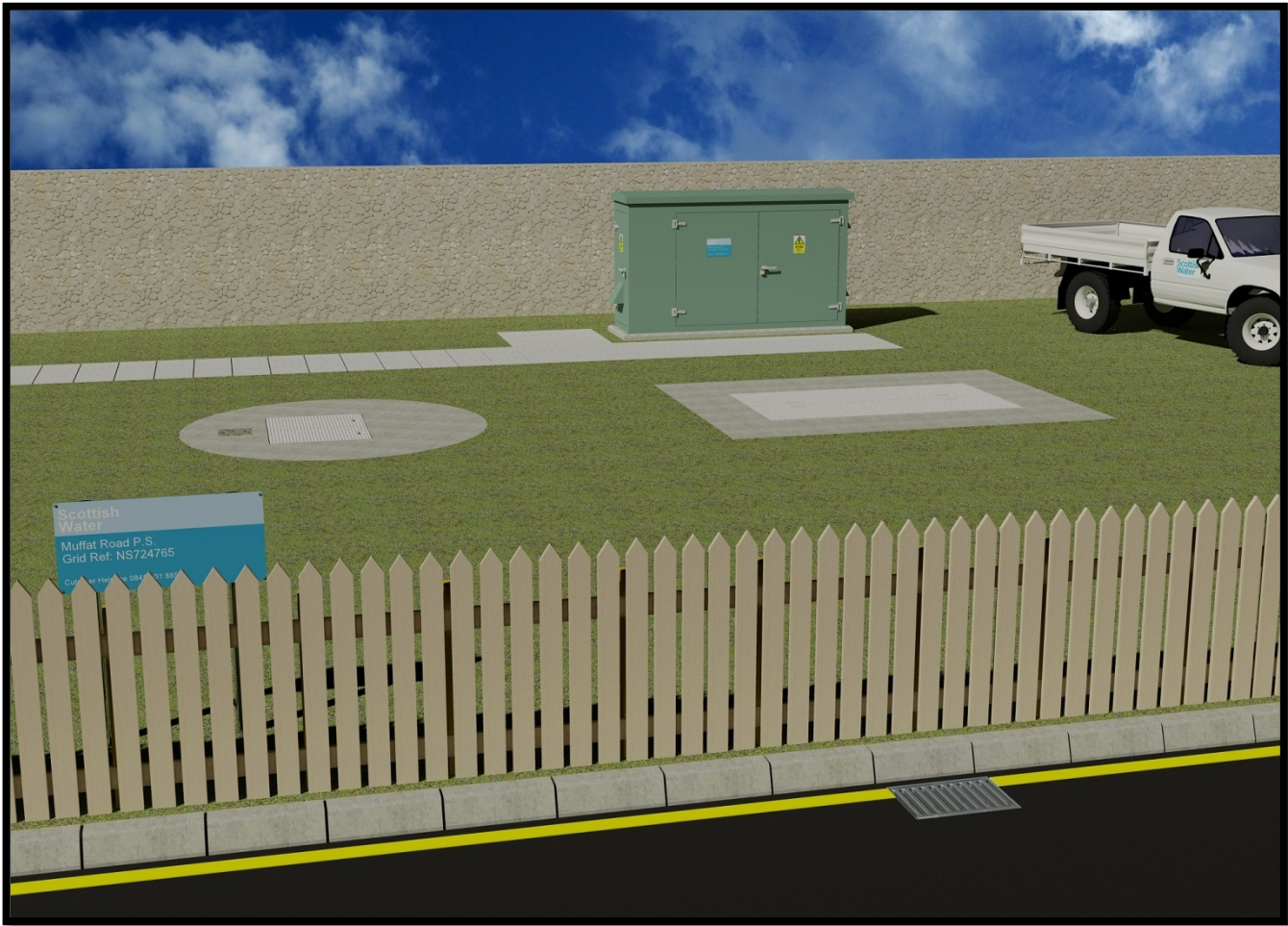
Site layout showing completed back filling; ready for commissioning (details omitted)
