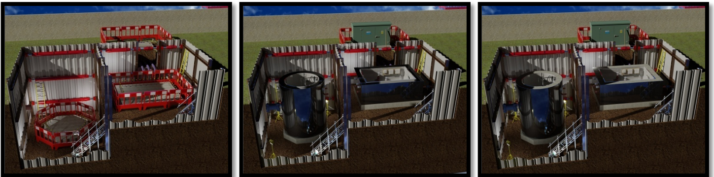
Installation of wet well and valve chamber, followed by pouring of concrete surround.
