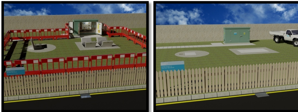
Installation of cover slabs, back fill and re-instatement of surrounding area.
