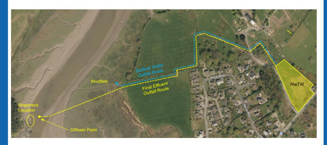
The surface water outfall pipe will terminate in the mudflat area of the River Urr and the final effluent pipe will terminate in a diffuser within the river as shown below.
