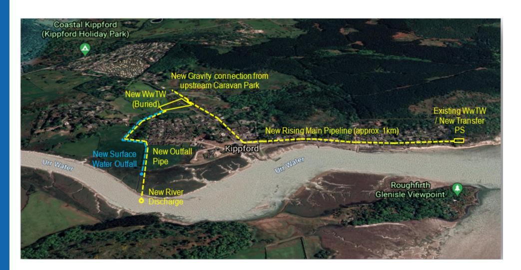
When the new infrastructure has been built, the existing WwTW will be converted into a new Pumping Station.
